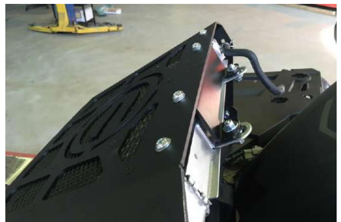
Install and tighten the relocation box
