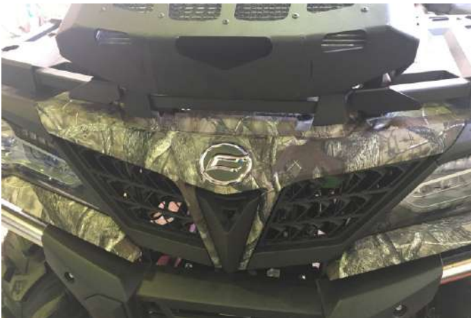
Install the grille
