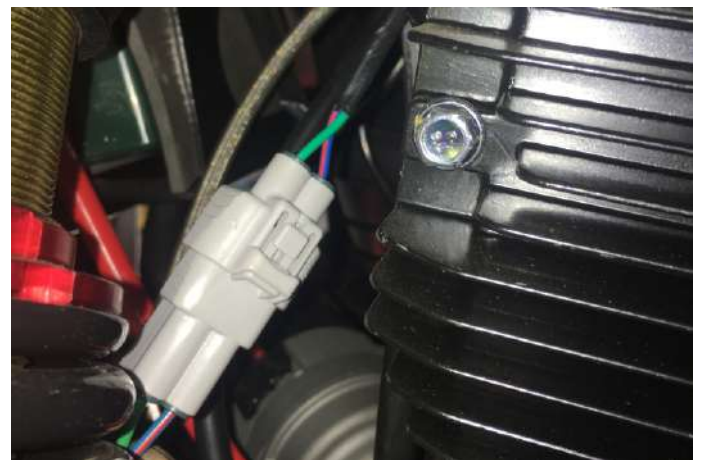
Disconnect the connector of the radiator fan
