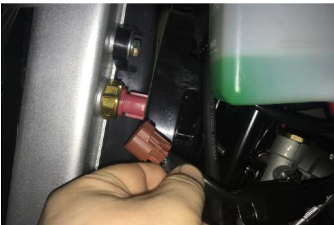
Unplug the temperature sensor connector
