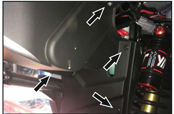
Remove the left back cover of the headlight
