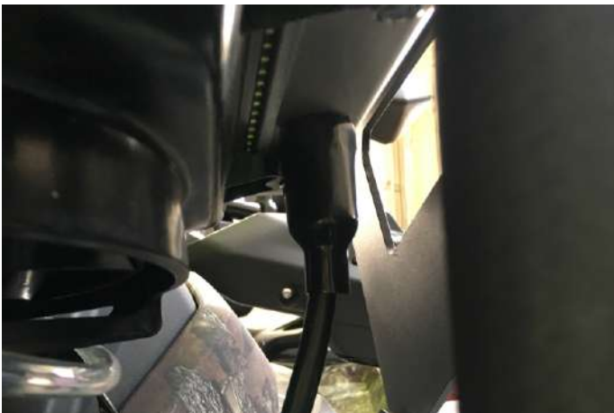
Plug the temperature sensor connector
