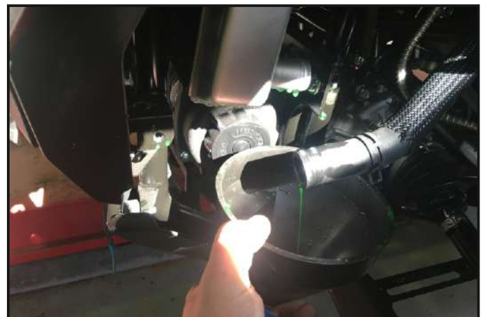
Remove the hose. Drain the antifreeze
