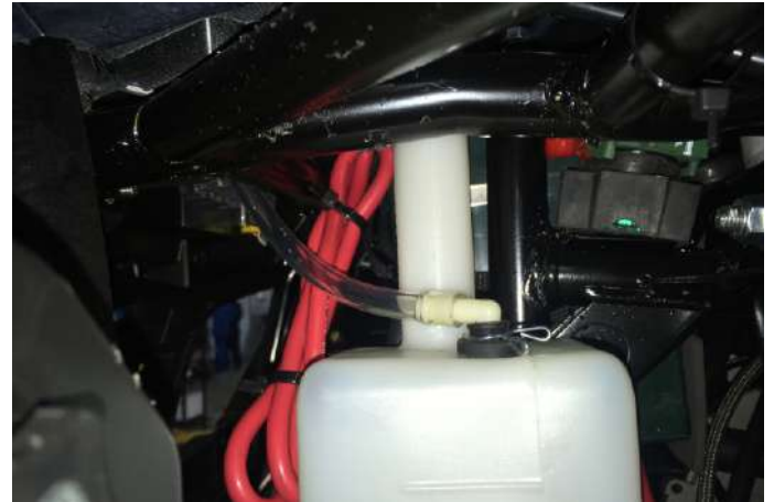
Install the radiator return tube to expansion tank
