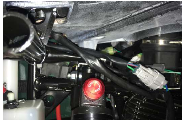
Connect the connector of the radiator fan
