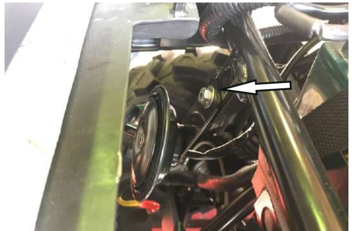
Install the horn on the frame
