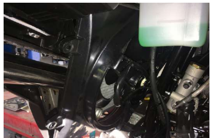
Remove the radiator fan to the left side
