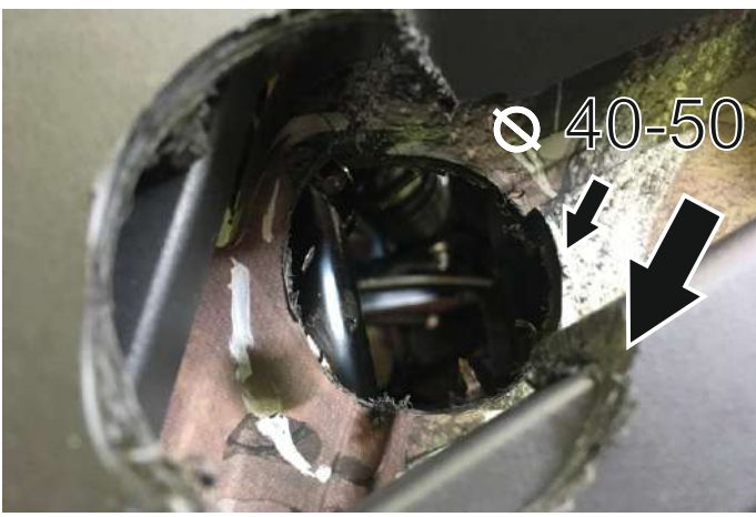
Drill a hole in front rack panel d40-50mm
