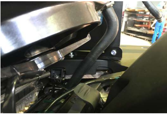
Install the bent hose on the radiator
