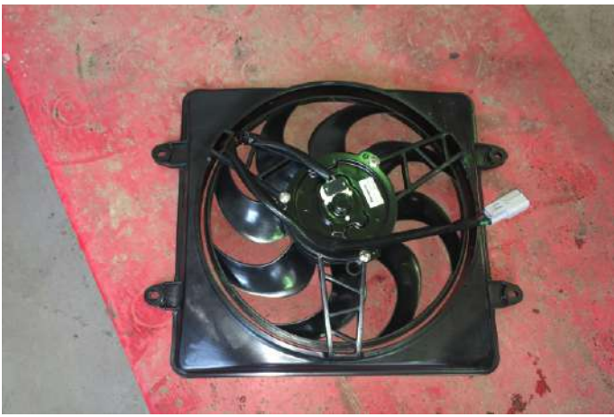
The radiator fan. Clean if needed.
