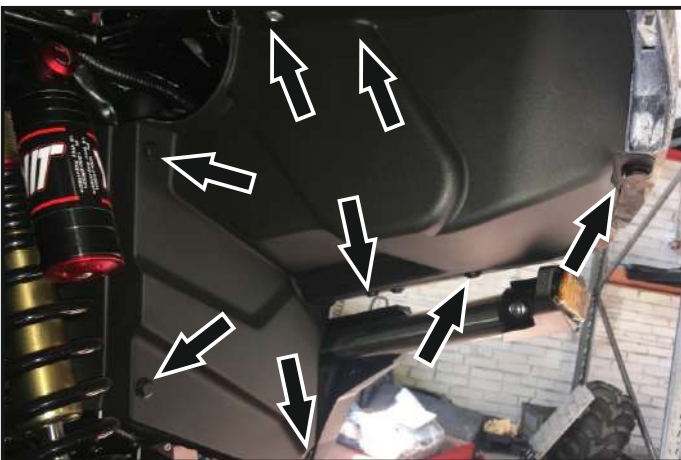
Remove the right back cover of the headlight
